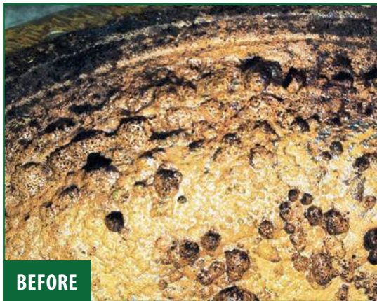
Heat exchanger floating head before and after pits in steel were filled using Novocoat EP3900 Machinable Paste . Novocoat SC5400 Tank Lining applied as topcoat.
