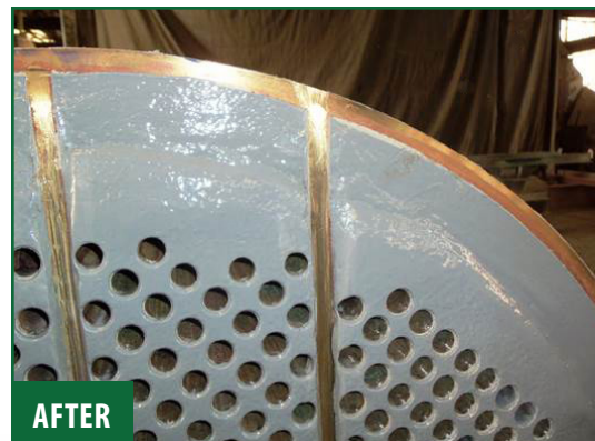
Tube sheet resurfaced using Novocoat EP5700 Ceramic Paste.
