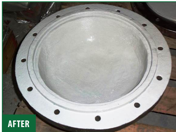
Heat exchanger floating head before and after pits in steel were filled using Novocoat EP3900 Machinable Paste . Novocoat SC5400 Tank Lining applied as topcoat.
